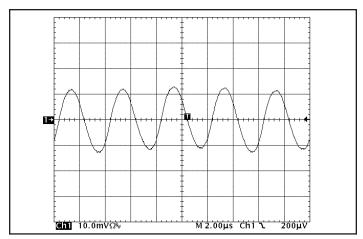
Figure 14: Input Terminal Ripple Current,  $i_{\mathcal{C}}$ , at full rated output current and nominal input voltage with 10 µH source impedance and 47 µF electrolytic capacitor (200 mA/div). See Figure 13.
