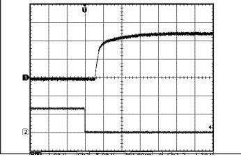
Figure 10: Turn-on transient at zero load (4 ms/div). Ch 1: Vout (1 V/div). Ch 2: ON/OFF input(5 V/div)
