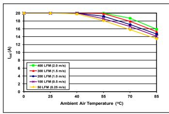
Figure 7: Maximum output power derating curves vs. ambient air temperature for airflow rates of 0 LFM through 400 LFM with air flowing lenghtwise from input to output (nominal input voltage).
