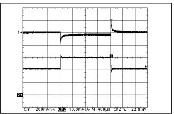
Figure 12: Output voltage response to step-change in load current (50%-75%-50% of lout(max): dI/dt = 5 A/ $\mu$ s). Load cap: 470  $\mu$ F, 30  $m\Omega$  ESR tantalum capacitor and 1  $\mu$ F cermaic capacitor. Ch 1: Vout (200 mV/div). Ch 2: lout (5 A/div)
