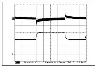
Figure 11: Output voltage response to step-change in load current (50%-75%-50% of lout(max);  $dI/dt = 0.1 \ A/\mu s$ ). Load cap:  $10 \ \mu F$ ,  $100 \ m\Omega$  ESR tantalum capacitor and  $1 \ \mu F$  cermaic capacitor. Ch 1: Vout (100 mV/div). Ch 2: lout (5 A/div)
