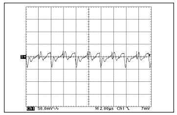
Figure 16: Output voltage ripple at nominal input voltage and rated load current (50 mV/div). Load capacitance: 1 µF ceramic capacitor and 10µF tantalum capacitor. Bandwidth: 20 MHz. See Figure 13.
