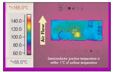
Figure 6: Thermal plot of converter at 20 amp load current with 55°C air flowing at the rate of 200 LFM. Air is flowing across the converter sideways from pin 3 to pin 1 (nominal input voltage).
