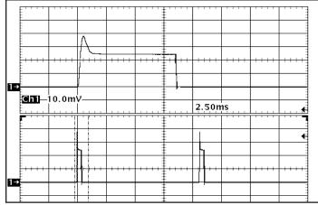
Figure 18: Load current (10 A/div) as a function of time when the converter attempts to turn on into a 10 m $\Omega$  short circuit. Top trace (2.5 ms/div) is an expansion of the on-time portion of the bottom trace.
